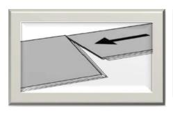
Install the second piece in the first row by laying the short end tongue onto the previously installed piece short-end groove.
