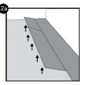
Disassemble the panels by lifting the short ends upward and disengage from the rest.
