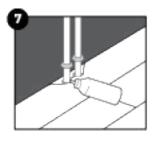
In case of a double pipe, drill a hole at each of the marked points that is equivalent to the diameter of the pipes plus 16mm. If located on the long side of the plank, make a 45 degree cut from each hole to the edge of the plank. Then, using an appropriate PVC glue along the cut edges of the piece you cut out, glue the piece in place. Be sure no glue comes between the cut out piece and the subfloor. For a perfect finish around pipes, use pipe covers.
