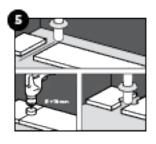
When sawing the panels make sure that the expansion gap under the door is 8mm. If you cannot lift the panel (e.g. under radiators), use the tapping block or pull-bar to tap the planks together.
