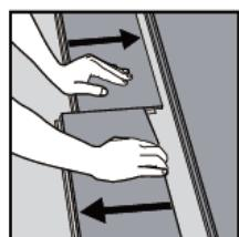
Separate the whole row by lifting it up delicately at an angle. To separate the planks, leave them flat on the ground and slide them apart. If planks do not separate easy, you can slightly lift up the planks (5°) when sliding them apart.
