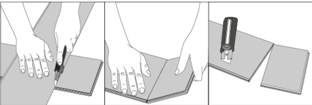
5. To cut the plank, use a simple utility knife and ruler, and with the top side facing up, cut heavily and several times on the same axis. The knife will not go through the surface but make a deep cut. You can then lift one half of the plank using your other hand to hold down the second placing it very close to the cut. The plank will split naturally.
