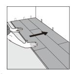
(7) After 2-3 rows. Adjust the distance to the front wall by leaving an expansion gap of 10mm (1/2"). Always ensure that the end joints are staggered at least 30cm (12"), both when in the same row as when from one row to the next one.
