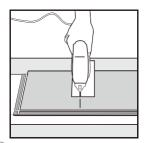
(4) If cutting with a jig saw, the laminate surface should be turned down. If cutting with a hand saw, the laminate surface should be face up.
