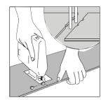
(9) Holes for pipes: measure the diameter of the pipe and drill a hole that is 20mm (7/8") larger. Saw off a piece as shown in the figure and lay the board in place on the floor. Then lay the sawed-off piece in place.
