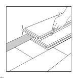
(8) To lay the last row: position a loose board exactly on top of the last row laid. Place another board on top, with the tongue side touching the wall. Draw a line along the edge of this boards, to mark the first board. Cut along the edge of this board to mark the first board. Cut along this line to obtain of the required width. Insert this cut board against the wall. The last row should be at least 50mm (2")wide. The spacers can then be removed.
