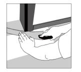
Door molding and skirting: lay a board (with the decorative side down) next to the door molding and as shown in the figure. Then slide the floorboard under molding.
