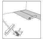
(1) After thoroughly cleaning the subfloor, you should install a foam underlay (unless your product has a pre-attached pad). Run the foam underlay in the same direction as the flooring planks. The underlay should be butted side-by-side with no overlap. Tape seams together. If you are installing over a concrete suboor, a 6-mil poly (plastic sheeting) is to be installed under the foam underlay. (Many foam underlays already have this plastic sheeting pre-attached).
