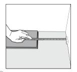
(3) At the end of the first row, leave an expansion gap of 10mm (1/2") to the wall and measure the length of the last plank to fit.
