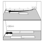
(5) Start the second row with the leftover cut part of the last plank of the previous row. This small plank should measure at least 30cm (12"). Otherwise, use another plank that should be cut in two. At any case, the short sides cut are distant from at least 30cm (12").
