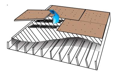
specifications to ensure adhesive is suitable for use over underlayment/industrial particle board sheeting. Countersink all screws/ nails and sand any uneven edges smooth. High spots should be sanded smooth and low spots shimmed with plywood that is secured to the sub floor and sanded flat.
