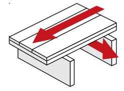
When installing the flooring in the same direction of the joists, a second layer of plywood is required to stiffen sub floor. Subfloor must be sheeted with ½" (15/32", 14mm) CD exposure 1 plywood sub floor panels. Use same method as attaching to solid board sub flooring.
