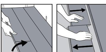
Separate the whole row by lifting it up delicately at an angle. To separate the planks, leave them flat on the ground and slide them apart. If planks do not separate easily, you can slightly lift up the planks (5°) when sliding them apart.
