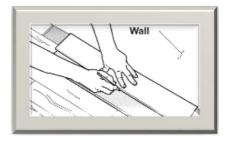
The last row (possibly the first row) plank width should be no less than 50mm (2") on the long seam. Remember to allow for a gap of 10mm (3/8") to the wall.
