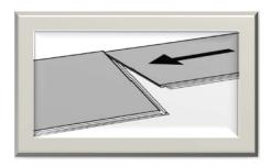
Install the second piece in the first row by laying the short end tongue onto the previously installed piece short-end groove.
