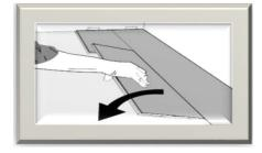
To install the remaining planks in the second row, first align the long edge tongue into the groove of the previous row at a shallow angle. Slide the piece to the left until the piece meets the previously installed piece.
