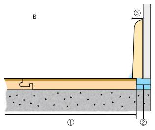
Movement joint x 1.5 = skirting board minimum thickness in mm
