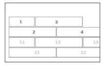
A. Products should be staggered in brick laid pattern; stagger equal to half of a plank for the first 2 rows, and then at least 18" for the following rows. Spacers should be placed against walls to maintain proper distance (1/4" - 1/2"). Tools needed: planks, underlayment, spacers.
